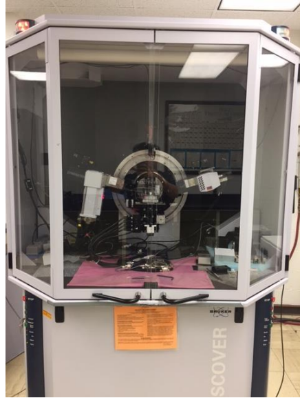
Figure 3.3.2: X-ray diffractometer (Bruker D8 Discover XRD, Cu k-alpha 1, 0.154 nm)
